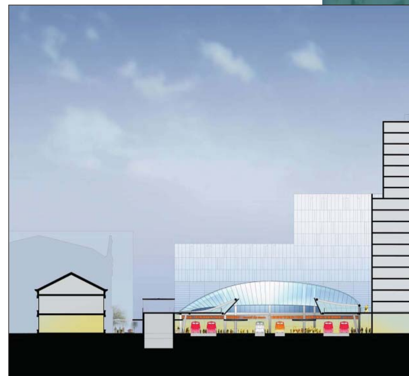
This section of Passenger Rail at approximately 18th Street shows bus access to the Regional Bus Facility.
